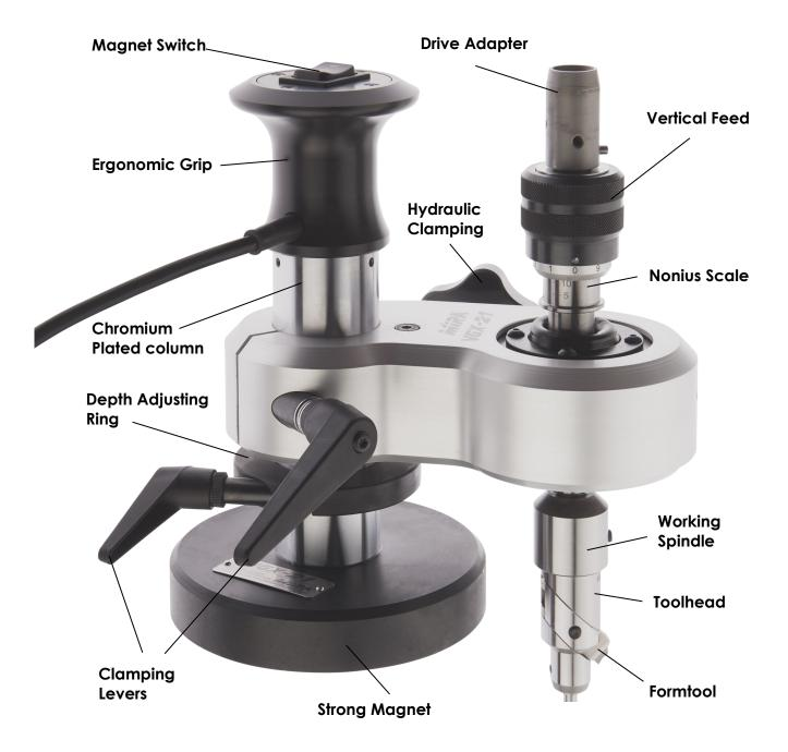
The portable VGX-21 valve seat refacing unit has been developed for the specialised petrol and diesel cylinderhead workshop. The highly accurate valve seat processing is achieved by a spherical spindle guide bearing as well as a unique **hydraulic ball clamping system**. A almost pressure free centering and braceless fixing of the MIRA® rotary head is made possible in order to achieve precise and concentric valve seats!
